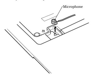
Figure 4-19 Removing the microphone
